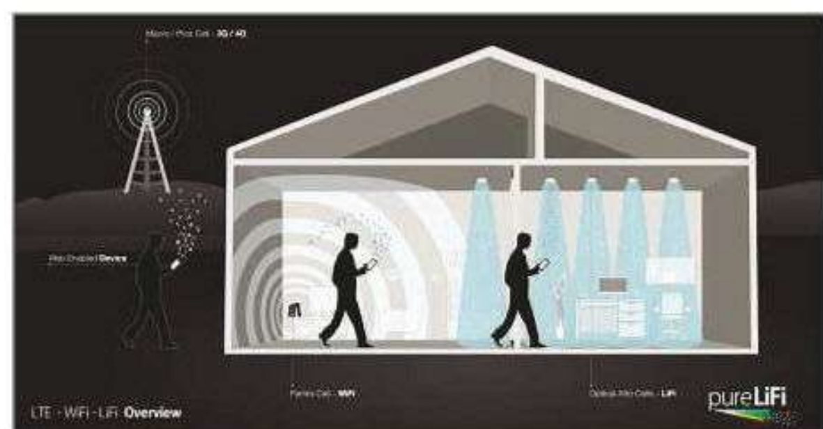
Li-Fi works by beaming data from LED bulbs to devices equipped with light receivers
